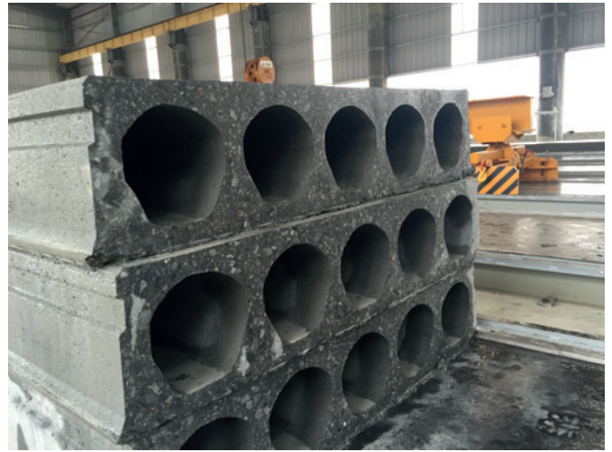
8 and 5 hole hollow core slabs. A point of note is the high quality of compaction at all points on the element
