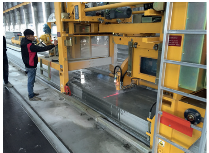
Multi-angle saw carrying out element cutting
