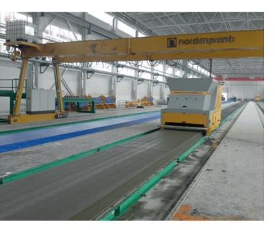
Nordimpianti proposed a number of measures to make operation easier and at the same time increasing the levels of worker safety: radio control for machine operation, laser positioning of machines, protection systems that can report production issues and even automatically stop the machine in cases of an emergency.
