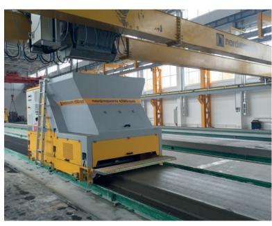
The Extruder in particular can be modified to change product height and product width according to a project's specification simply by changing the forming inserts enabling slab widths of 1000, 1200 and 1500 mm wide to be produced.
