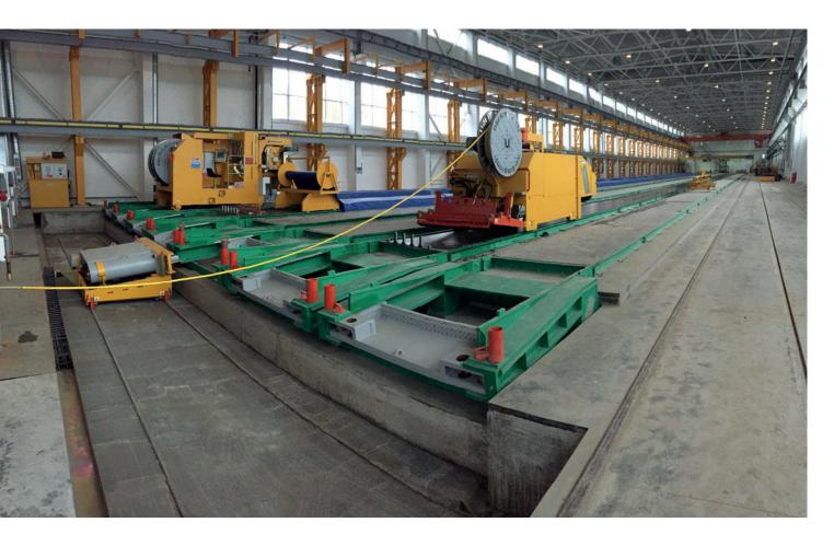
The new production hall has 7 hollow core slab production beds, each 114 meters long. This means a potential productivity of up to  $270,000 \text{ m}^2$  per year.
