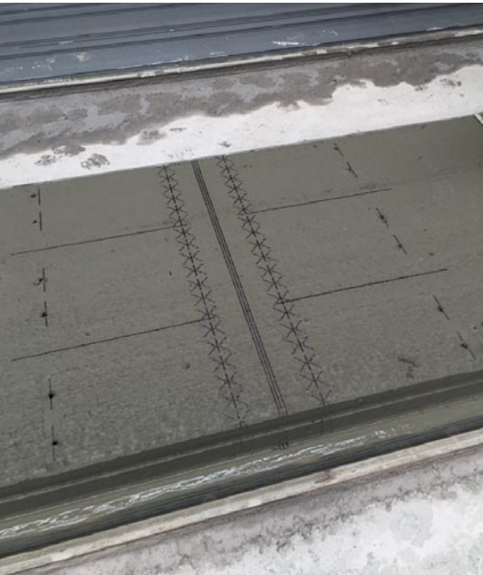
Example of production data printed by the plotter on the hollow core slabs.
