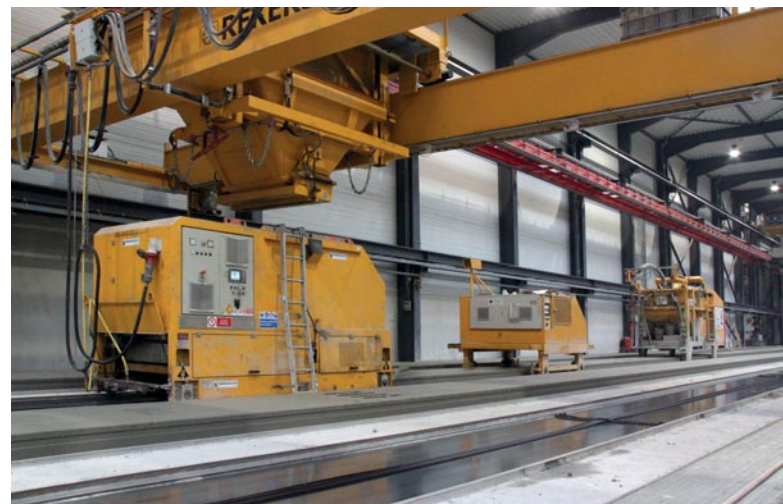
The work sequence showing the completely automatic concrete distribution, the extruder in the casting phase and a plotter for the traceability of the final product.
