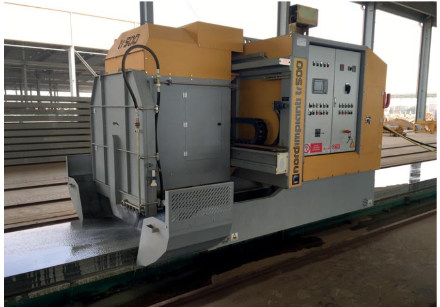
Automatic cutting saw with laser positioning device.
