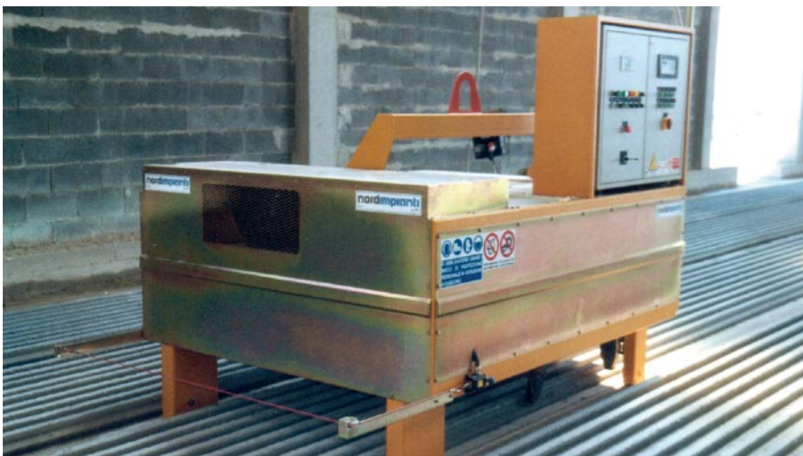
The plotter marking elements on the production bed.
