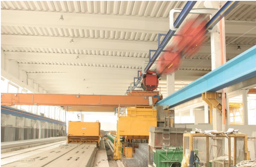
Fly bucket transporting the concrete automatically from the batching plant to the casting machine on the production bed.
