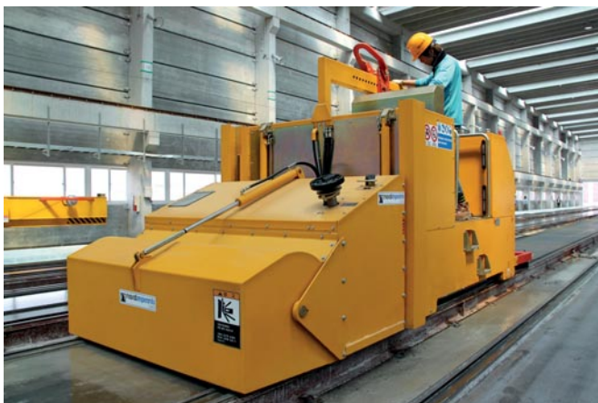
The multifunction bed cleaner cleaning and oiling the production bed ...
