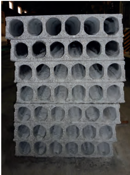
High level of hollow core slab geometry attained from the Nordimpianti Extruder.
