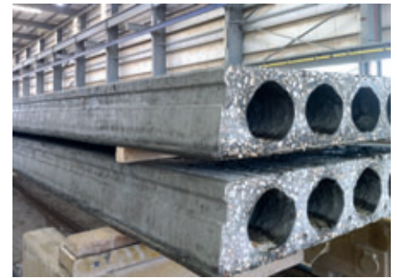
View showing the high quality finish of the side profile achieved by Nordimpianti's Extruder machine on 900 mm wide hollow core slabs.
