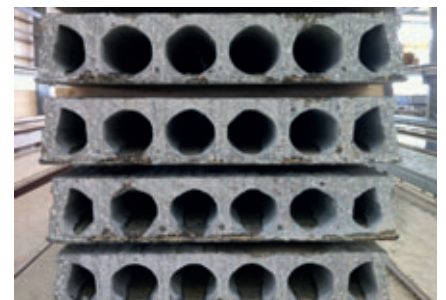
1100 mm wide hollow core slabs produced by a Nordimpianti Extruder.
