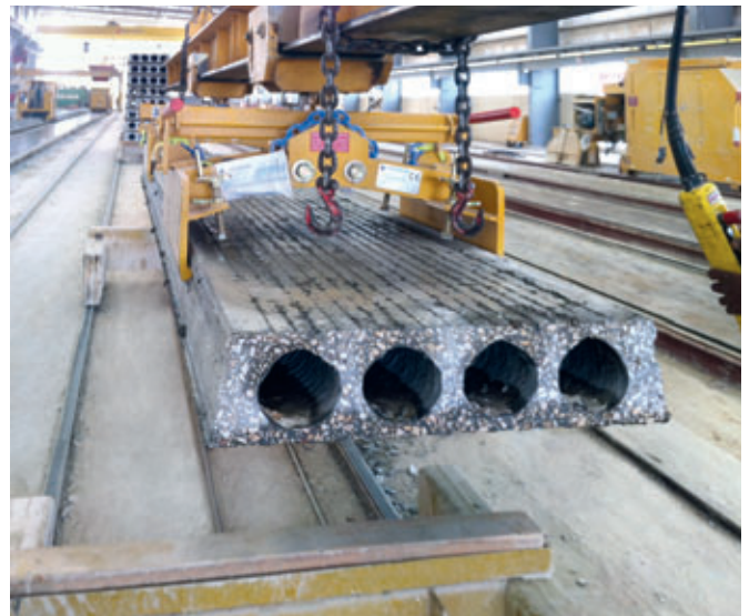
Lifting of a 900 mm hollow core slab using dedicated clamps.
