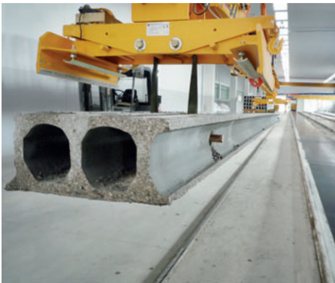
Removal of a hollow core slab from the production bed using a lifting beam.
