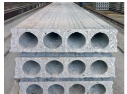
900 mm wide hollow core slabs produced by a Nordimpianti Extruder.
