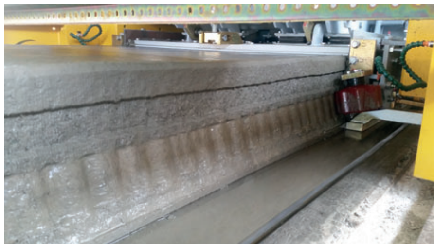
Detail of the innovative side edge rail developed by Nordimpianti.
