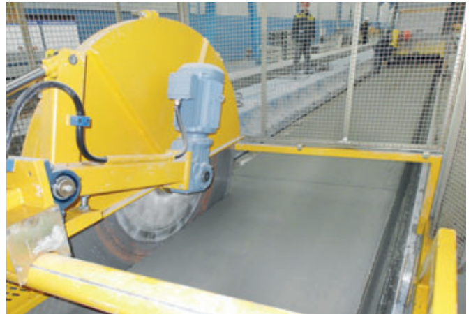
Longitudinal cutting on a hollow core slab, still in its fresh concrete state, using Nordimpianti's fresh concrete saw.
