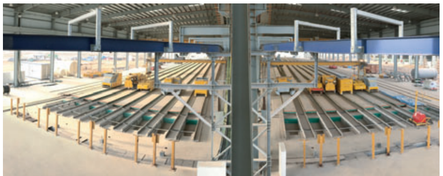
View of 2 production areas each having 8 x 165 m production beds at the factory in Jizan.
