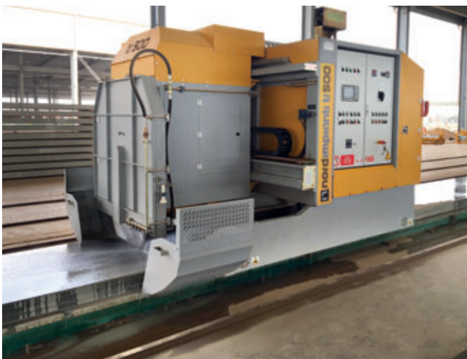
The Automatic version of the 500 TR Transversal Saw during the cutting of hollow core slabs on the production bed.
