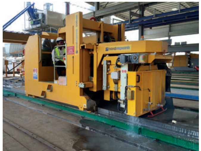
The 500 AM Multi Angle Saw cutting hollow core slabs on the production bed.
