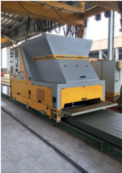
Nordimpianti's EVO Extruder during casting of the 150 mm high hollow core slabs.
