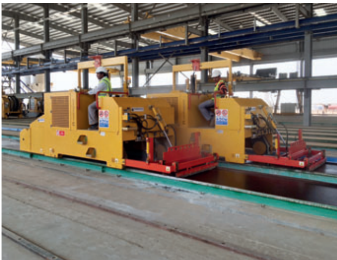
The Multi-Function Bed Cleaner cleaning the production bed.
