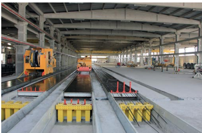
Interior view of the new production area for hollow core slabs in the Kambeton prefabrication factory.
