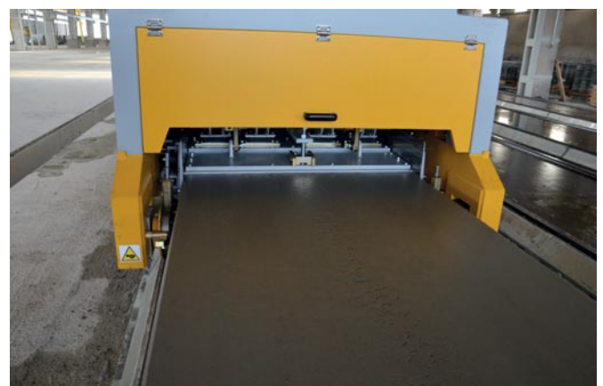
The Nordimpianti EVO e120 Extruder, capable of producing hollow core slabs with heights of 150, 200, 265, 320, 400 and 500 mm.
