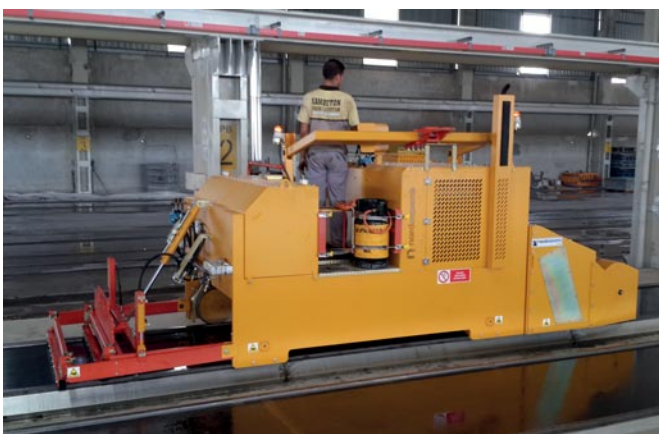
Multi-function bed cleaner during production bed preparation.
