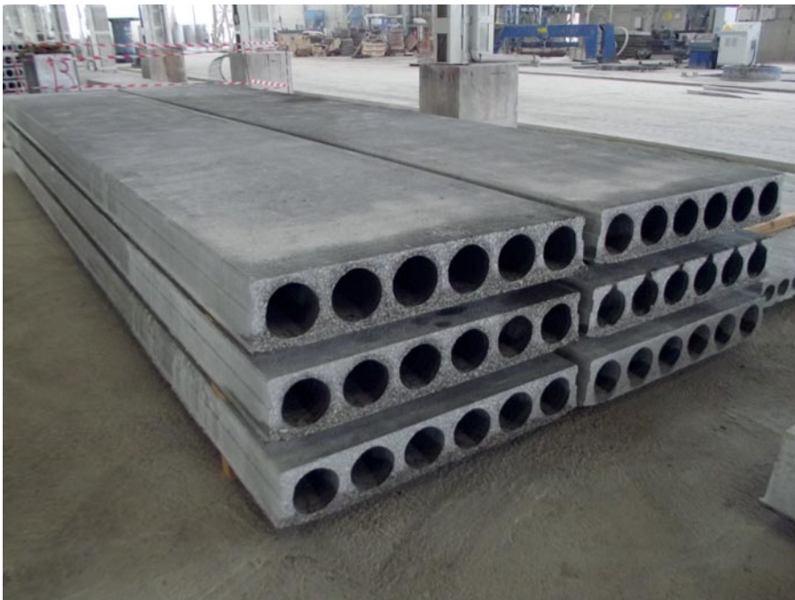
The very first produced hollow core slabs, one still on the production bed, ready to be supplied for on-site assembly.
