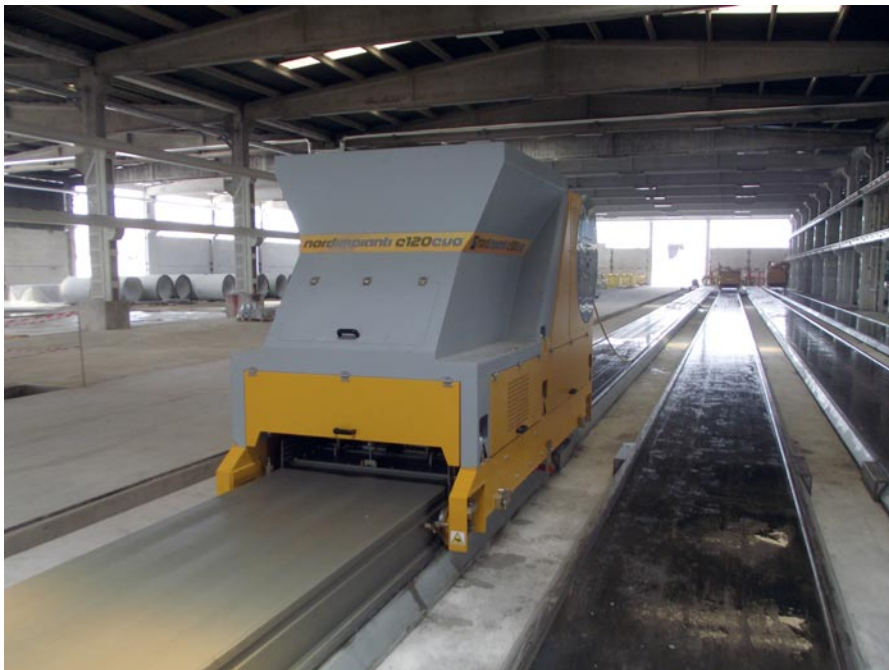
Hollow core slab immediately after production, demonstrating the high concrete compaction achieved by Nordimpianti's Extruder machine.
