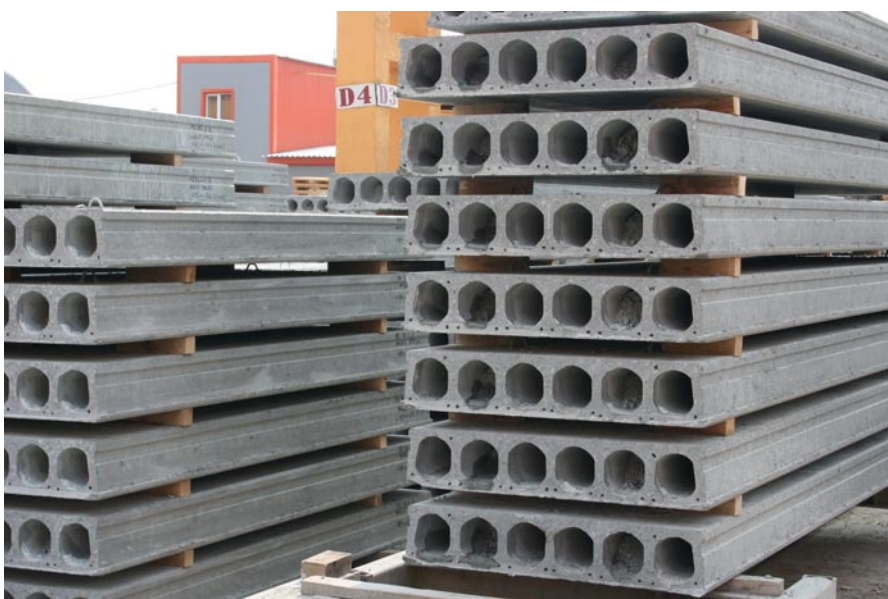
1200 mm wide hollow core slabs produced on 1500 mm production beds.
