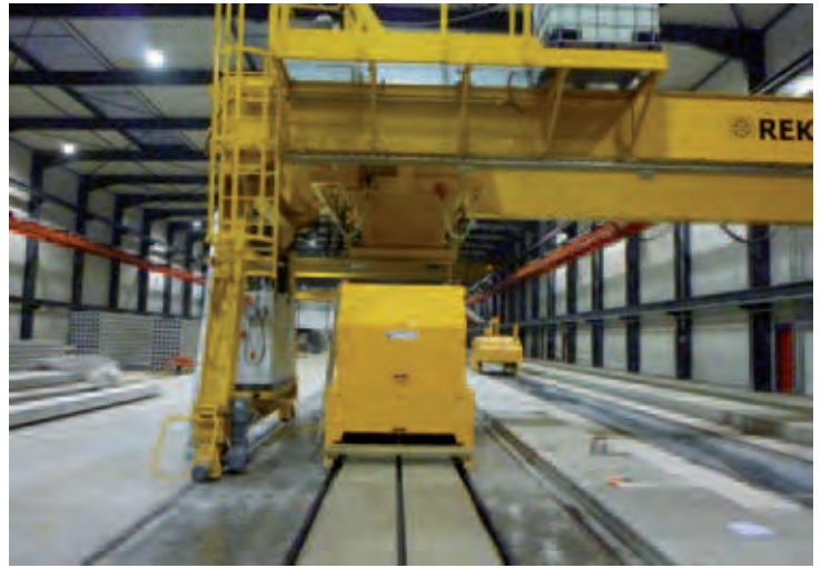
The Nordimpianti Extruder EV2000 showing its ability to cast a single 1200mm wide element or two 600mm wide panels.
