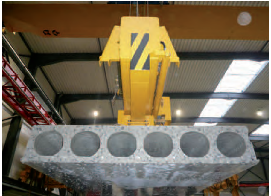
Excellent concrete element quality achieved with Nordimpianti's Extruder machine and the use of quality aggregates.
