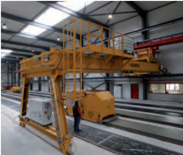
The Nordimpianti Extruder EV2000 showing its ability to cast a single 1200mm wide element or two 600mm wide panels.
