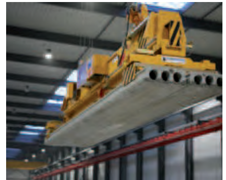
Single 1200mm or two 600mm elements being transported by telescopic lifting beams from Nordimpianti
