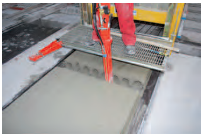
The new Concrete Aspirator designed to remove the semi-dry concrete worked by the Extruder after compaction.
