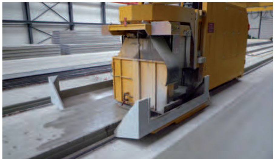
The Nordimpianti Saw 500AM that can cut concrete panels up to 520 mm high
