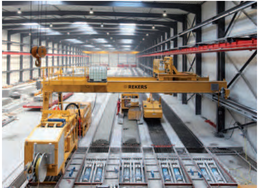
The plant has 2 production lines, each consisting of 5 production beds, 120 m long.
