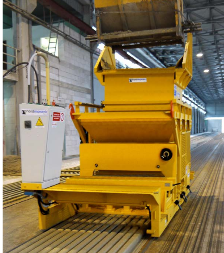
Wet Casting wf machine
