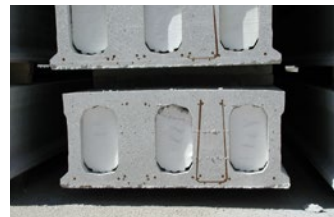
POSSIBILITY TO HAVE TRANSVERSAL STEEL REINFORCEMENT
