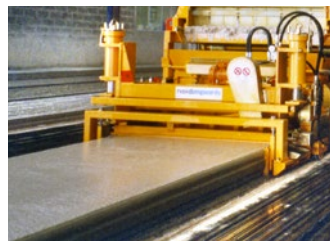
Hollow core wall panel with coloured aggregate finish
