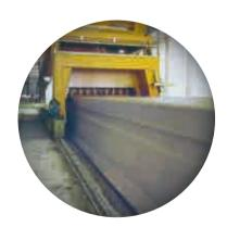
**Performance** Production of prestressed concrete elements with heights up to 1000 mm.
