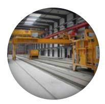
Manufacturing plant with fixed casting beds and movable machines that can be configured for small or large production to meet the needs of your company.
