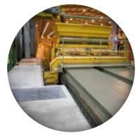
Special carousel plant with movable casting beds and fixed machinery for high output production requiring only the minimum of personnel.
